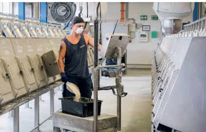
The chemicals used for vulcanization are stored in closed containers. When opened, automatic extraction is activated. CMR substances were substituted.
